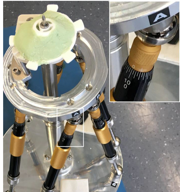
Fig. 2 The Jig-Maker with the surgical template on top of the upper platform. Adjusting the length of all struts enables pose-setting with respect to the alignment pin in the central axis of the device, which represents the planned trajectory
